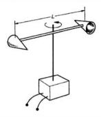
$B = 10^{-4}$  T at this point. Find the maximum voltage induced by a wind of speed v = 100 km/h, assuming that the cups rotate at exactly this speed.
